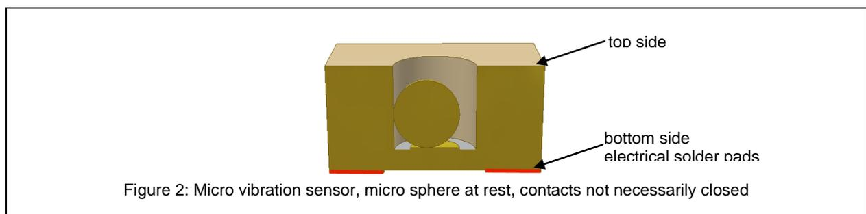
The unidirectional sensor version MVS1006.01 is open at rest, when mounted in upside down position, so that the micro sphere is on the top side of the sensor, which has no contact pad.
